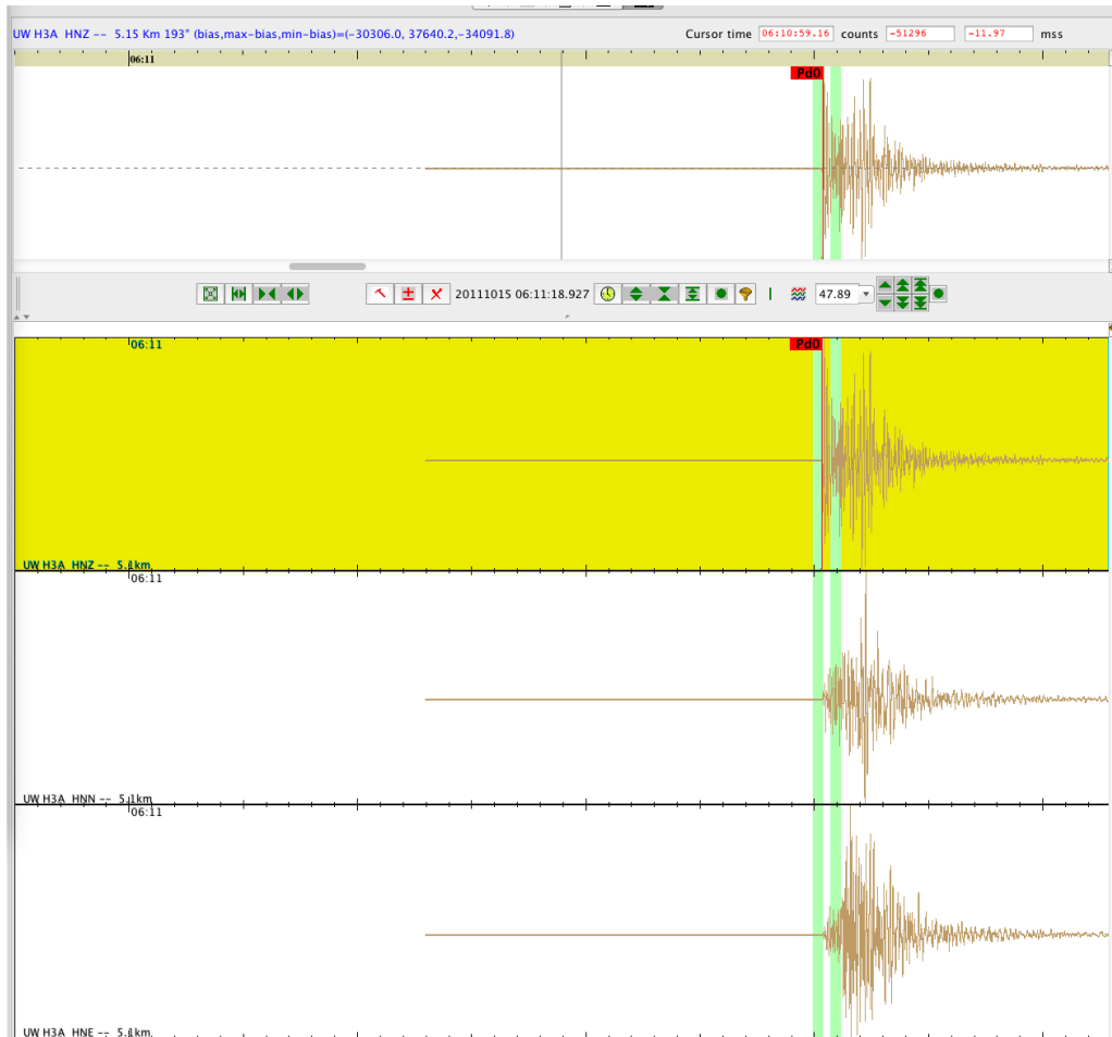
Figure 6.1 Screen shot of analyst’s view of the data from the 15 October, 2011 M_c 3.4 Wooded Island swarm earthquake recorded at HSN station H3A. Red label “flags” attached to thin red bars reveal time of analyst-reviewed phase picks, labeled with pick type and weight. These records verify that shaking levels were not close to levels that might be expected to cause damage, but of a level sufficient to be felt rather sharply.
